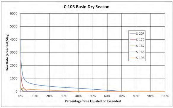
Figure C-23. Flow duration curves for the C-103 basin water control structures during the dry season.
