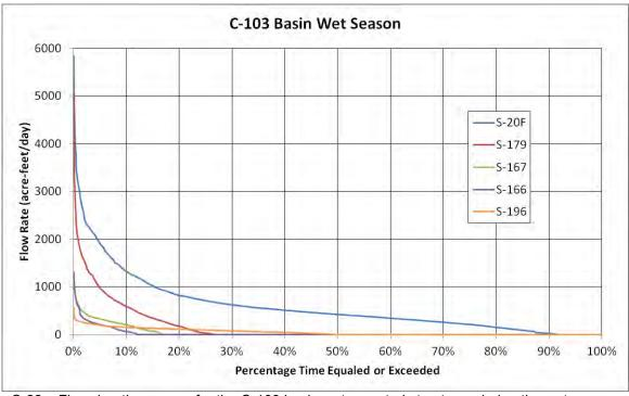
Figure C-22. Flow duration curves for the C-103 basin water control structures during the wet season.
