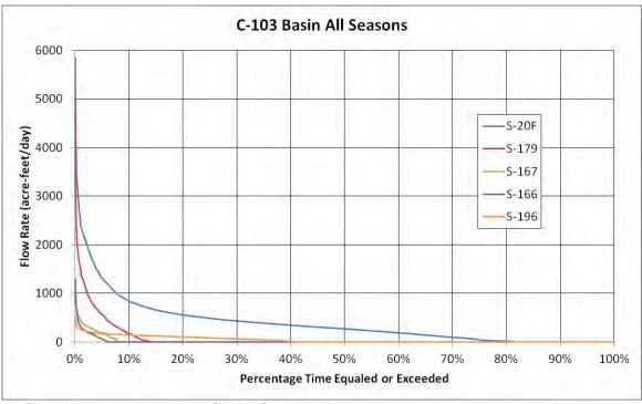
Figure C-21. Flow duration curves for the C-103 basin water control structures during all seasons.
