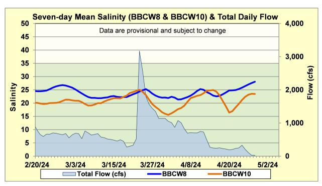
**Figure BB-1.** Seven-day mean salinity at BBCW8 and BBCW10 and total daily flow in Biscayne Bay. Total daily flow was calculated using flow from structures S20G, S20F, S21A, S123, and S700P.
