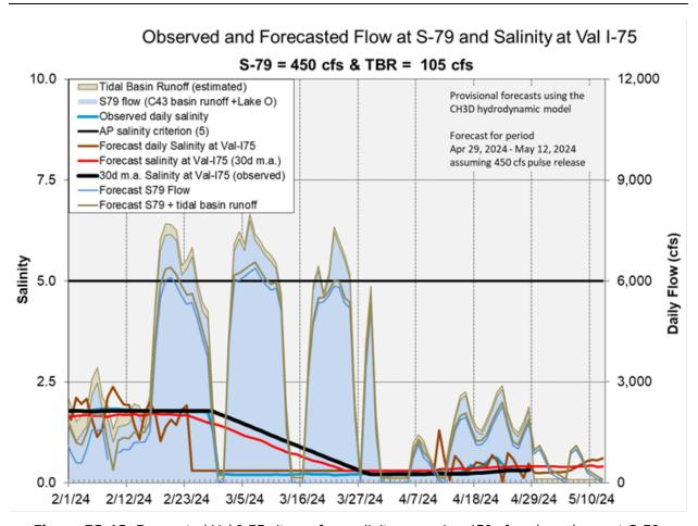
**Figure ES-13.** Forecasted Val I-75 site surface salinity assuming 450 cfs pulse release at S-79.
