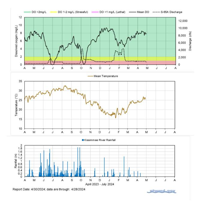
**Figure KB-6.** Kissimmee River channel mean daily dissolved oxygen concentration (mg/L), S-65A discharge (cfs), temperature (°C) and rainfall (inches). Dissolved oxygen (DO) and temperature are mean daily values averaged for PC62, KRDR02, KRBN, PC33, PC11, PD62R, and PD42R with an average of six stations reporting this week. Rainfall values are daily totals for Kissimmee River (Pool BCD) AHED watershed.
