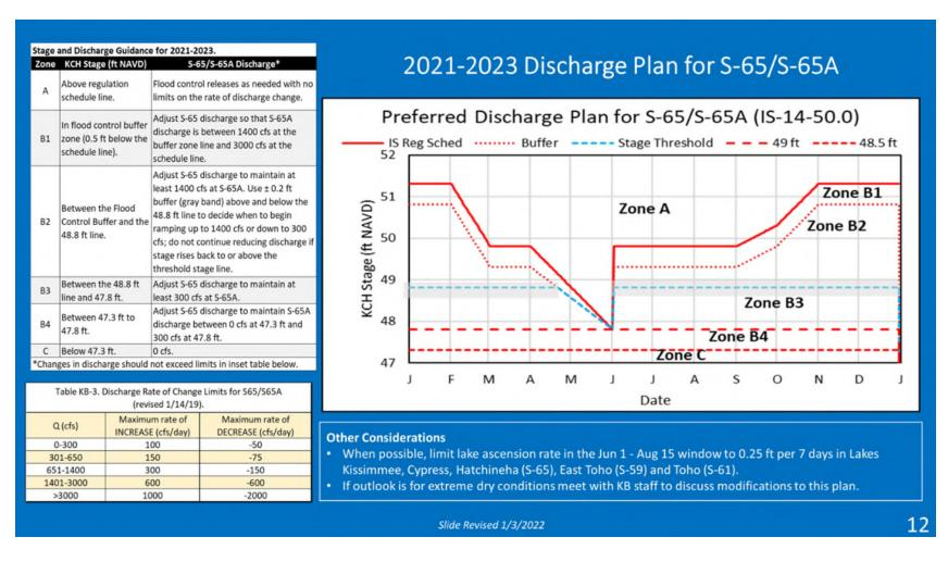
Figure KB-8. IS-14-50 Discharge Plan for S65/S65A with discharge rate of change limits (revised 1/14/19).
