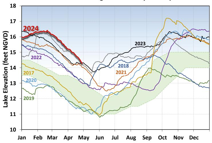
**Figure LO-3.** The current and eight prior year's annual stage hydrographs for Lake Okeechobee in comparison to the recovery envelope (light green). A shift from the normal ecological envelope to the recovery envelope occurred because the 30-day minimum lake stage (elevations exposed for at least 30 days, nonconsecutively) in the June 1 – July 31, 2023 window was >13 ft NGVD29 (11.75 ft NAVD88).
