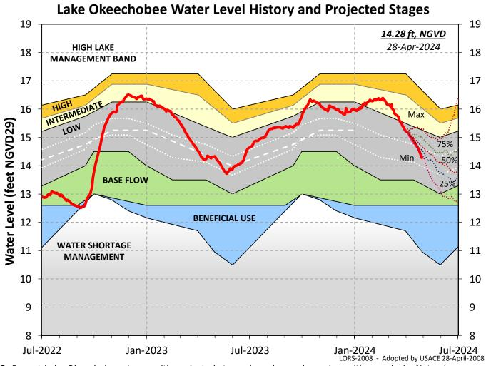
Figure LO-2. Recent Lake Okeechobee stages with projected stages based on a dynamic position analysis. Note stages are in NGVD29.
