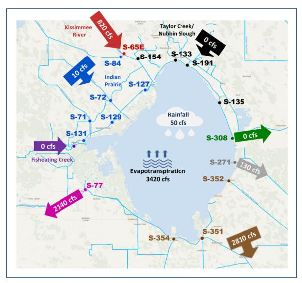
**Figure LO-5.** Inflows into Lake Okeechobee from Indian Prairie basins, Taylor Creek/Nubbin Slough, Kissimmee River and Fisheating Creek, and outflows to the west via S-77, to the east via S-308, to the south via S-351, S-352, S-354, and to southeast via S-271 (formerly Culvert 10A) for the week of April 22 - 28, 2024.
