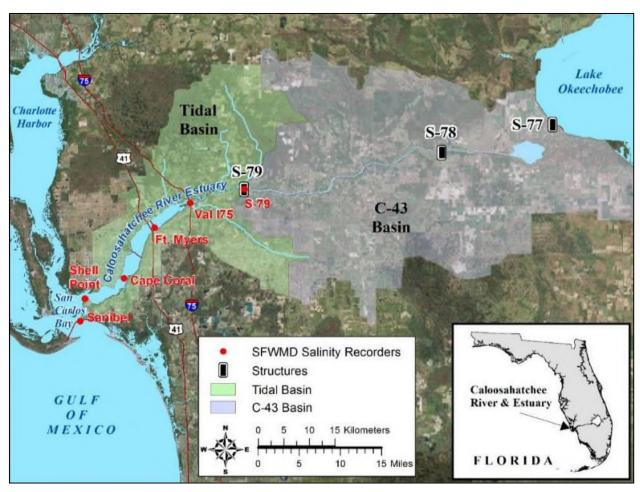
**Figure ES-6.** Basins, water control structures and salinity monitoring sites in the Caloosahatchee River Estuary.
