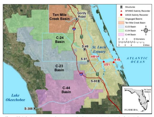
Figure ES-1. Basins, water control structures and salinity monitoring sites in the St. Lucie Estuary.
