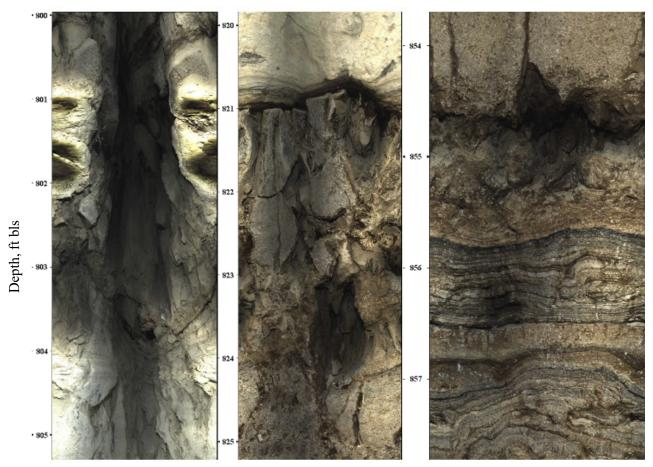
Figure 11. APhpz-1 flow zones as shown in these images from the OBI log. From left to right, a large vertical solution-enhanced fracture from 800 to 805 ft bls; a zone of fractured rock bounded on the top by an open bedding plane solution zone from 820 to 825 ft bls; and bedding plane solution, vertical fractures, and contorted, laminated bedding with bedding plane solution from 854 to 857.5 ft bls.
