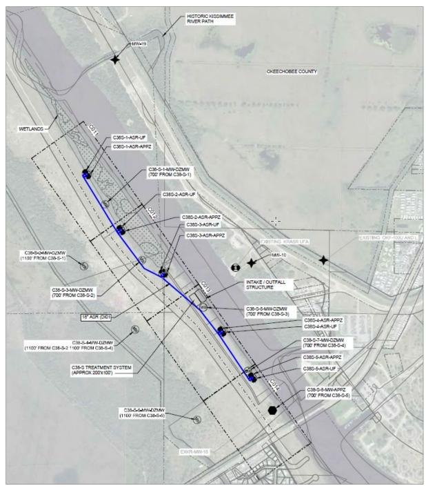
**Figure 5-1**. Conceptual layout of the C-38S ASR wellfield.
