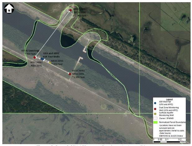
**Figure 3-2**. C-38N ASR test well and monitoring well layout.
