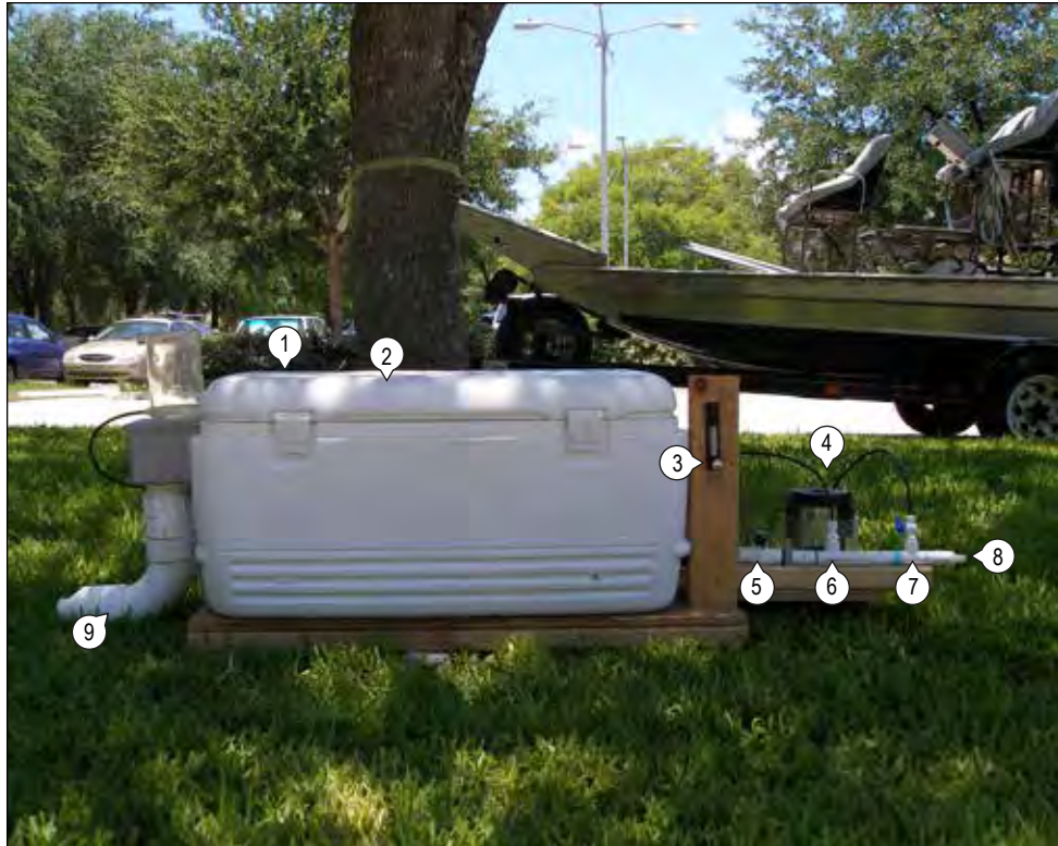
Figure 1-10. The outer flow-through chamber, flow rate controls and connections for the multiprobe attachment fittings.
