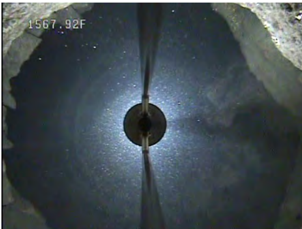
Figure 9. Clean and clear open hole at 1,568 ft bpl.
