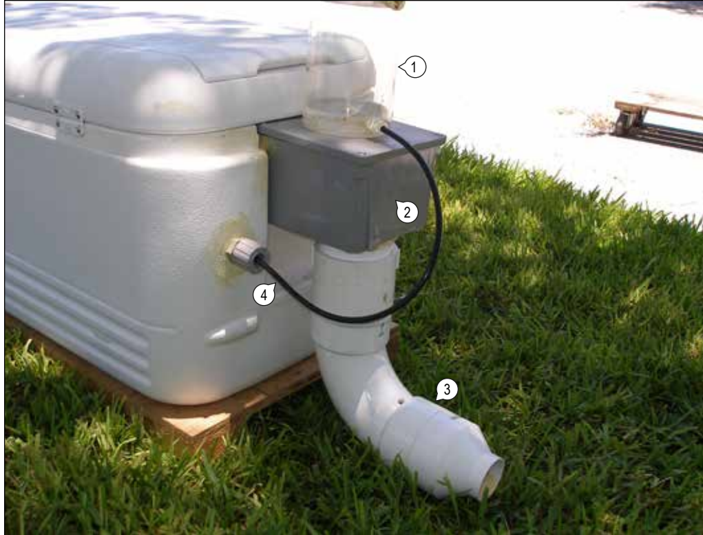
Figure 1-12. The outer flow-through chamber discharge and multiprobe fittings.
