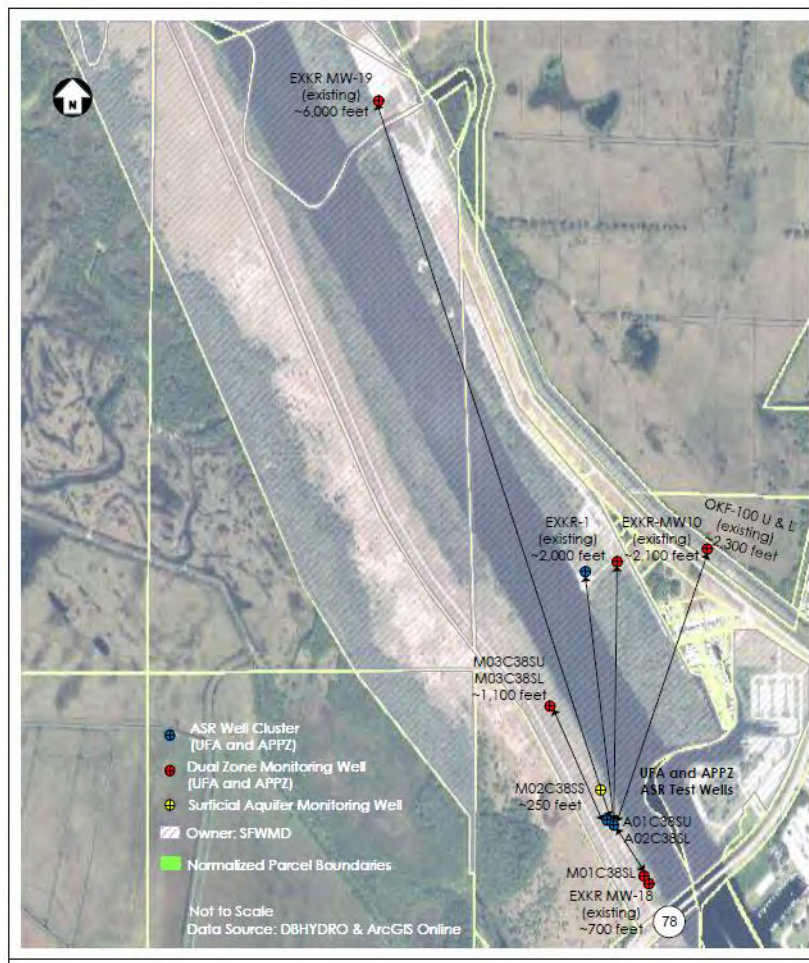
Figure 5. C-38S General ASR System Site Layout
