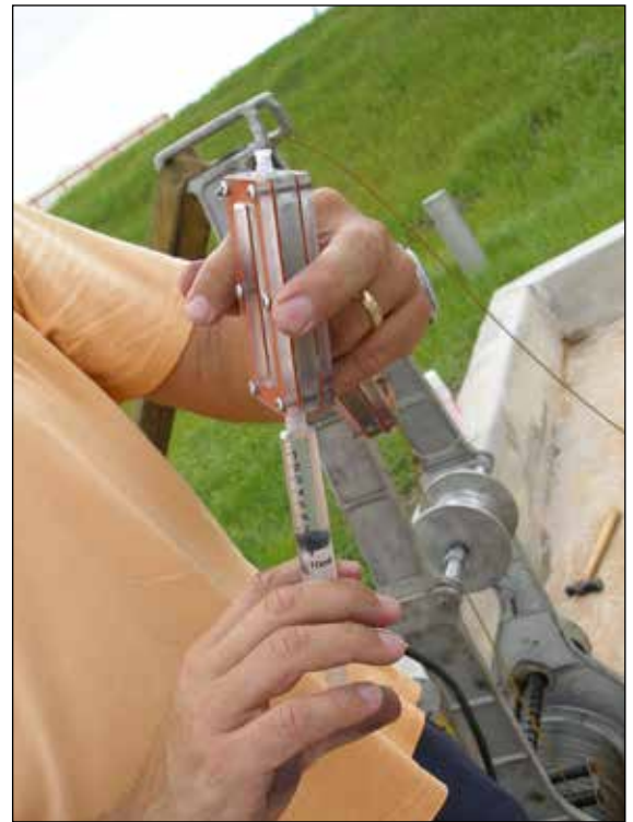
Figure 1-3. Loading a diffusion chamber with a culture of bacteria using a syringe.
