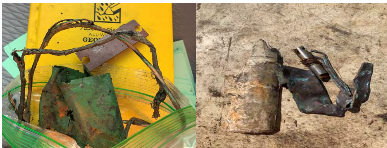
Figure 7. Recovered XY caliper tool and PVC drop pipe pieces.
