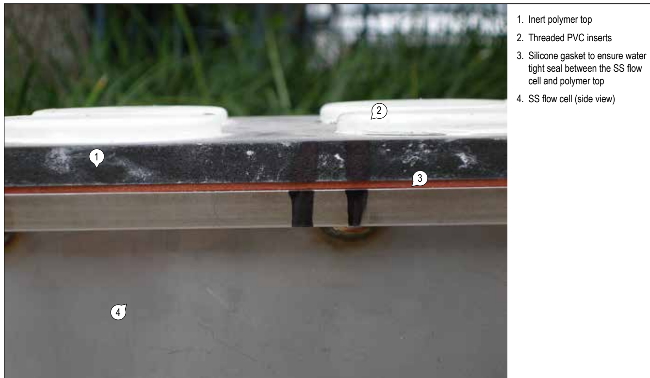
Figure 1-8. The stainless steel flow-through chamber showing the silicon gasket that seals the connection between the polymer top and the stainless steel chamber (side view). This gasket prevents the source water in the outer flow-through chamber from leaking into this chamber.
