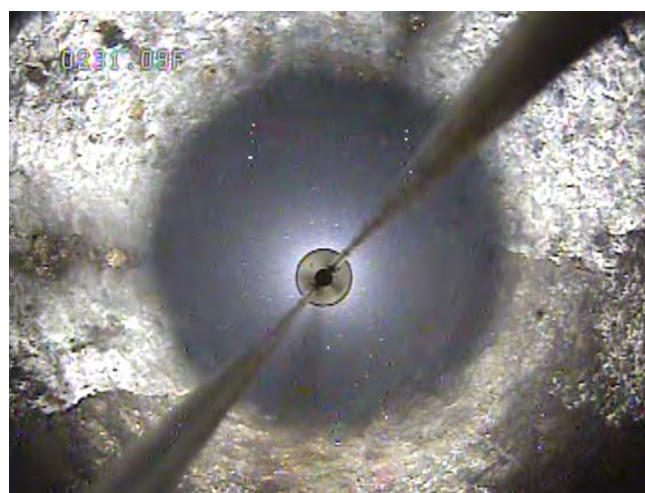
Figure 2. Black encrustation at 629 ft bpl. Figure 3. White encrustation at 231 ft bpl.
