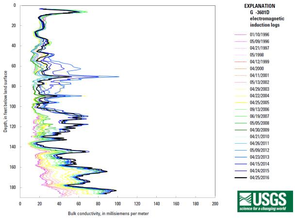
Figure D-25. Induction logs for monitor well G-3601D (190 feet deep) in North Miami, northeastern Miami-Dade County (From: Valderrama 2017).
