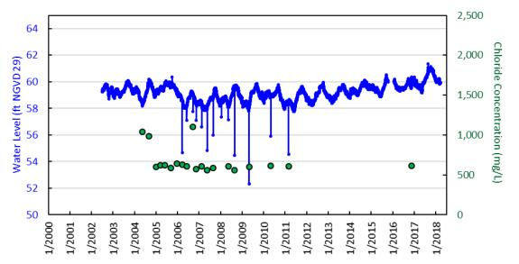
Figure D-36. Water levels and chloride concentrations in Upper Floridan aquifer monitor well G-2618 (1,164 feet deep), western Broward County.
