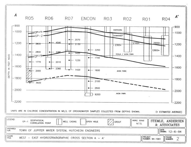
Figure D-42. Hydrogeologic cross-section of Town of Jupiter Floridan aquifer system wells RO1 to RO7 (From: Stemle, Andersen & Associates, Inc. 1994).
