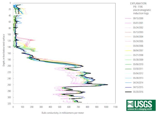
Figure D-15. Induction logs for monitor well PB-1195 (325 feet deep) in Boynton Beach, southeastern Palm Beach County (From: Valderrama 2017).
