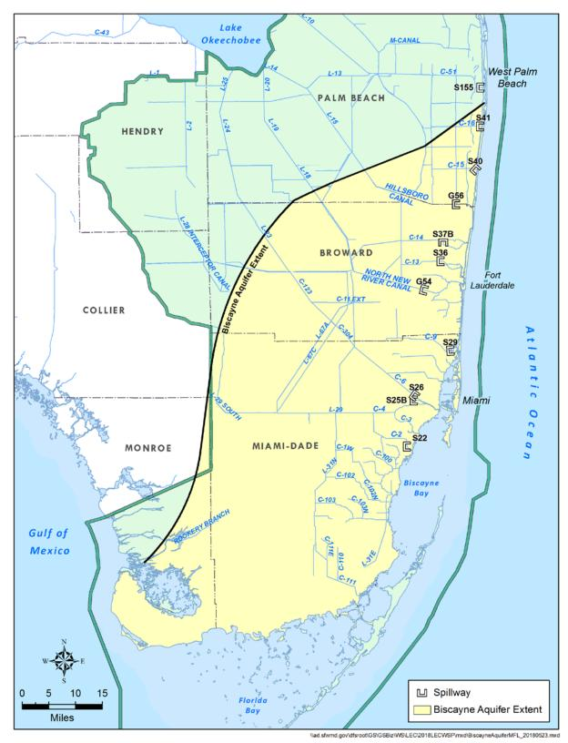
Figure C-7. Biscayne aquifer Minimum Flow and Minimum Water Level water management structures.
