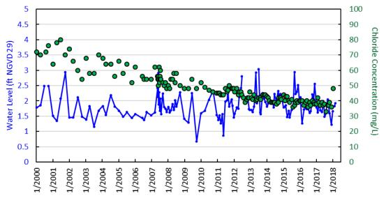
Figure D-27. Water levels and chloride concentrations in monitor well G-354 (92 feet deep) in Hialeah, northwestern Miami-Dade County.
