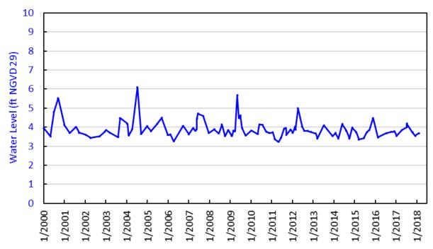
Figure D-3. Water levels in the surficial aquifer system at well G-617 (29 feet deep) in Davie, central Broward County.
