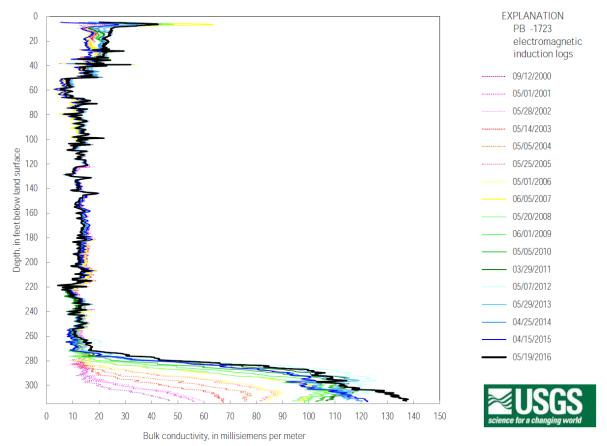
Figure D-14. Induction logs for monitor well PB-1723 (318 feet deep) in Lake Worth, eastern Palm Beach County (From: Valderrama 2017).
