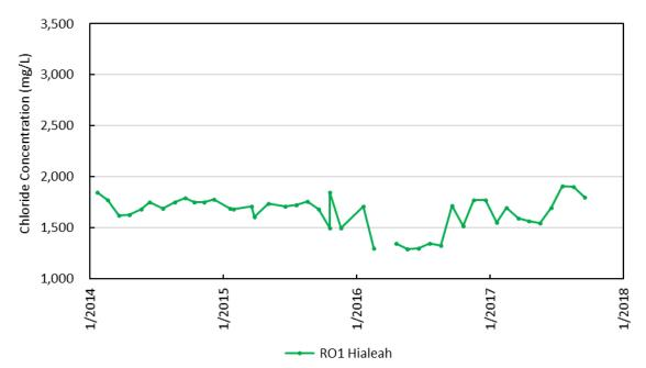
Figure D-49. Chloride concentrations in Miami-Dade Water and Sewer Department Floridan aquifer system (Upper Floridan aquifer) well RO1 Hialeah.
