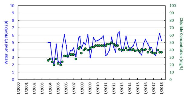
Figure D-20. Water levels and chloride concentrations in monitor well G-2693 (229 feet deep) in Hillsboro Beach, southeastern Broward County.
