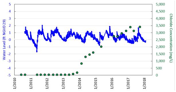
Figure D-31. Chloride concentrations in monitor well TPGW-7D (114 feet deep) in Homestead, southeastern Miami-Dade County.
