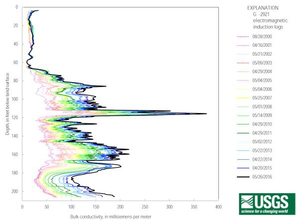
Figure D-22. Induction logs for monitor well G-2921 (206 feet deep) near Davie, southeastern Broward County (From: Valderrama 2017).
