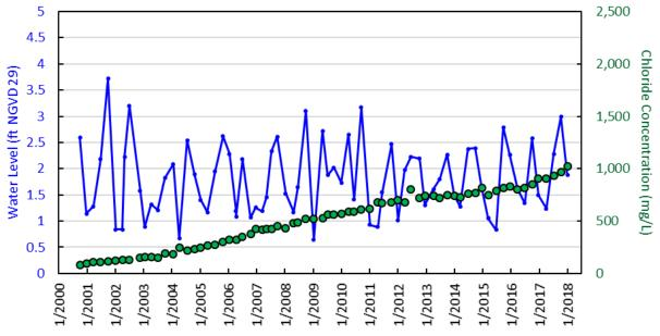
Figure D-21. Water levels and chloride concentrations in monitor well G-2899 (165 feet deep) in Fort Lauderdale, eastern Broward County.
