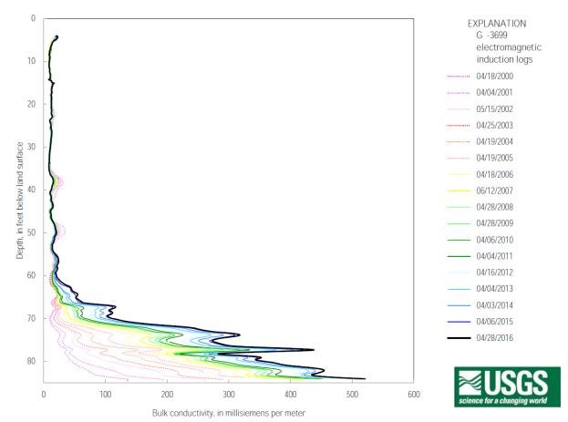
Figure D-30. Induction logs for monitor well G-3699 (88 feet deep) near Homestead, southern Miami-Dade County (From: Valderrama 2017).
