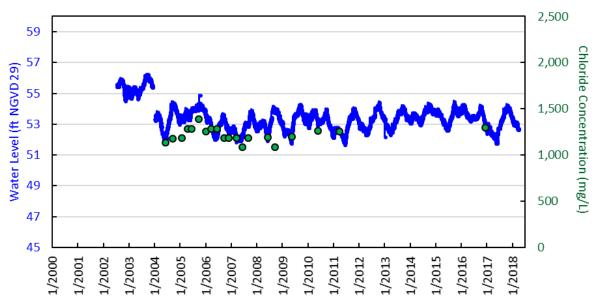
Figure D-35. Water levels and chloride concentrations in Upper Floridan aquifer monitor well PBF-7U (1,447 feet deep), western Palm Beach County.
