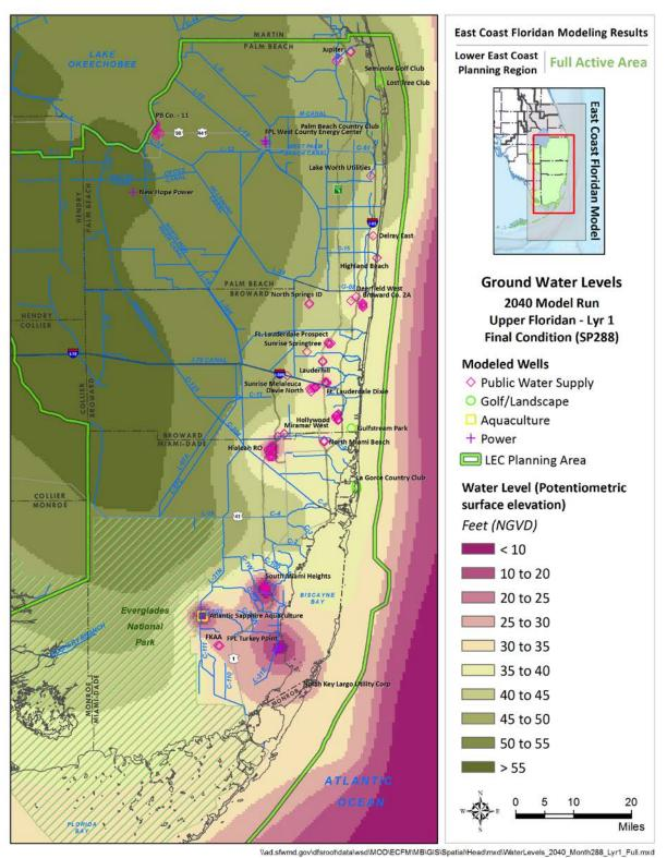
Figure D-55. Final water levels in 2040 in the Upper Floridan aquifer (Layer 1).
