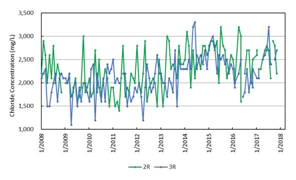
Figure D-41. Chloride concentrations in Village of Tequesta Floridan aquifer system (Avon Park Permeable Zone) wells 2R and 3R.
