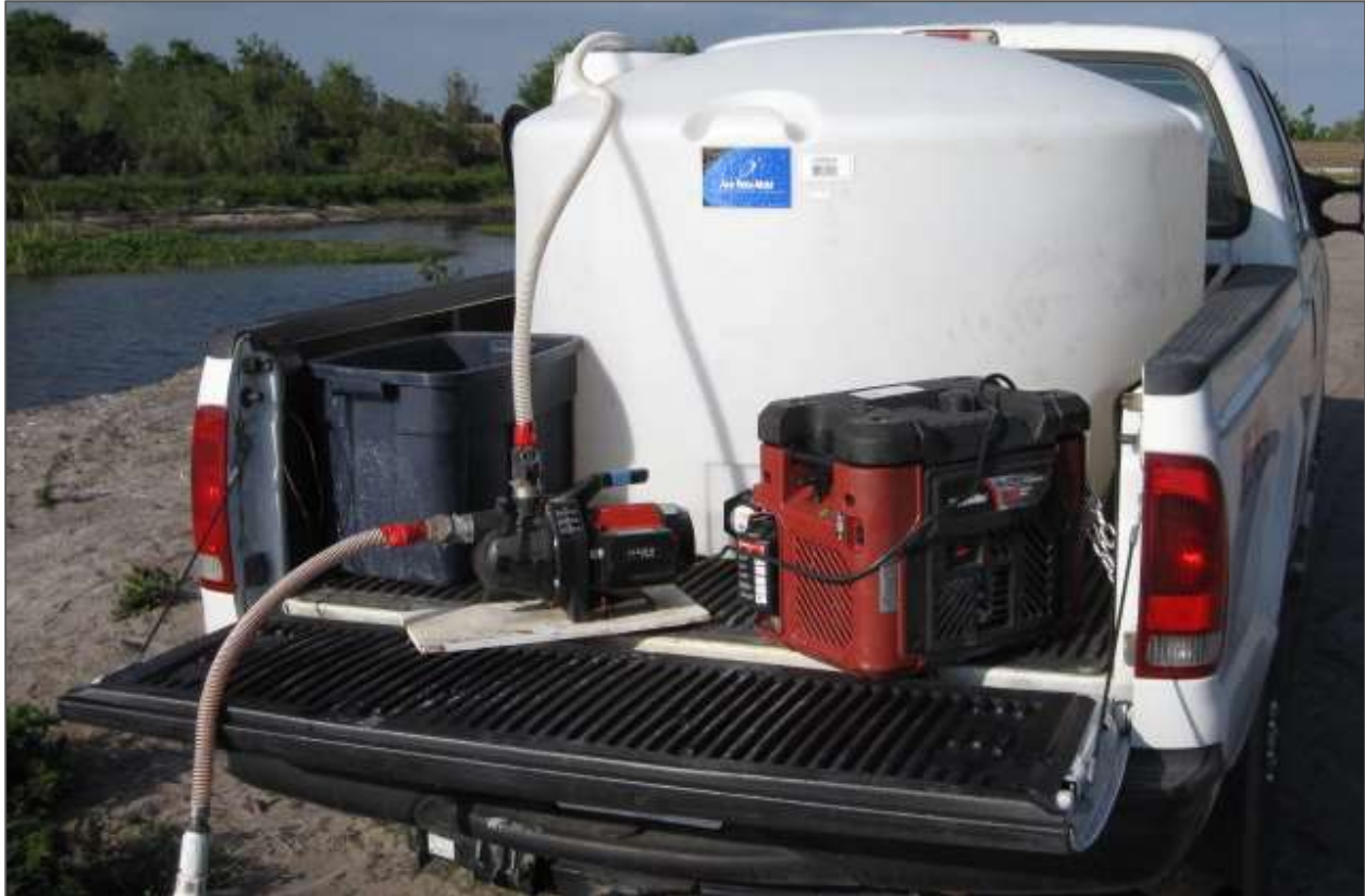
Figure 5. Recharge Water Collection System
