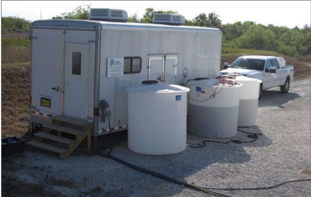
Figure 4. Example Exterior of Mobile Laboratory and External Holding Tanks with Exterior Access to Pump House
