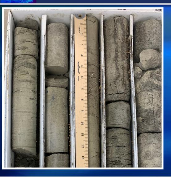
Goal: to chemically analyze the core from ASR L63N to find areas of potentially high metal concentrations using a hand held X-Ray fluorescence (XRF).
