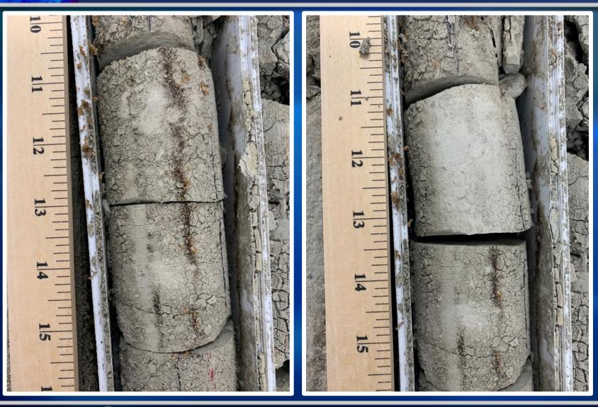
Debris and rust were cleaned off of the core surface using a wire brush before every analysis.
