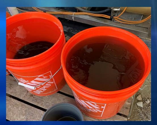
Solids settling after 90 minutes (Left: ceramic Aqua Aerobic, Right: polymeric Suez)
