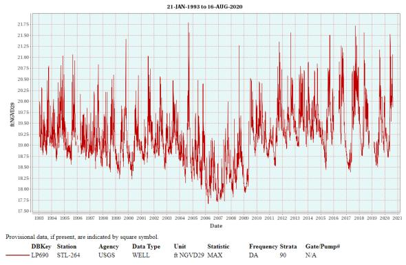
Figure 6-5. Water levels in surficial aquifer system monitor well STL-264, north central St. Lucie County.
