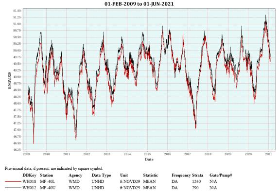
Figure 6-12. Water levels in Floridan aquifer system monitor wells MF-40U and MF-40L, north central Martin County.
