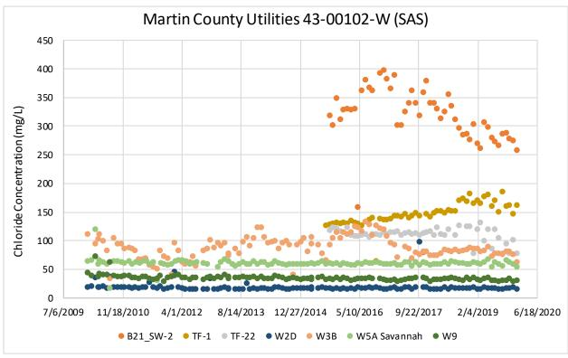
Figure 6-6. Chloride concentration trends at surficial aquifer system wells monitored by Martin County Utilities.
