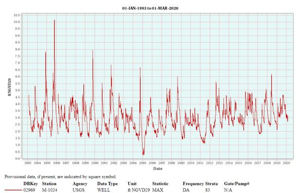
Water levels in surficial aquifer system monitor well M-1024, southern coastal Figure 6-2. Martin County.
