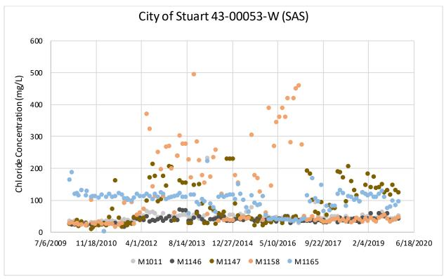
Figure 6-8. Chloride concentration trends at surficial aquifer system wells monitored by City of Stuart.
