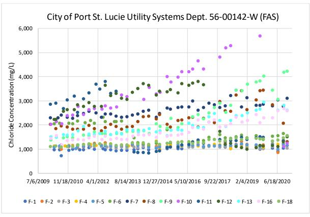
Chloride concentration trends at Floridan aquifer system wells F-6, F-9, and F-10 to Figure 6-17. F-12 (open to the Upper Floridan aquifer) and wells F-1 to F-5, F-7, F-8, F-13, F-16, and F-18 (open to the Upper Floridan aquifer and Avon Park permeable zone) monitored by the City of Port St. Lucie Utility Systems Department.
