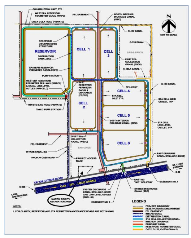
Figure 7-4. C-44 reservoir and stormwater treatment area cells.
