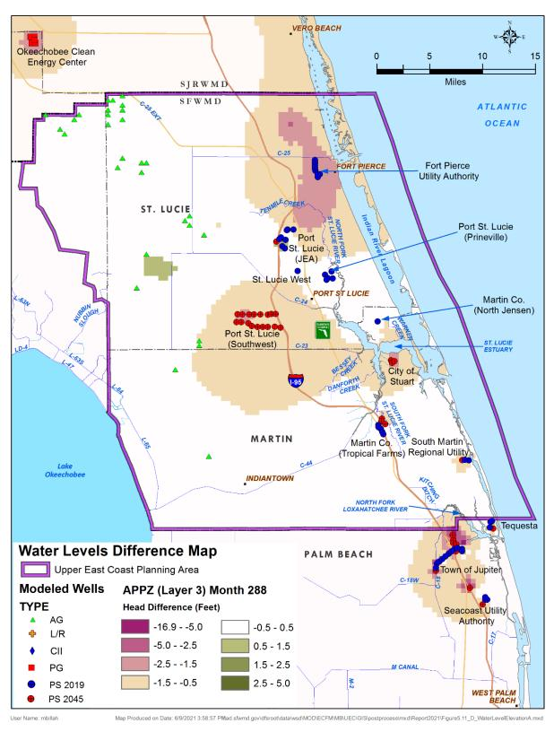
Figure 6-19. Water level changes (head difference) in the Avon Park permeable zone between 2019 and 2045.
