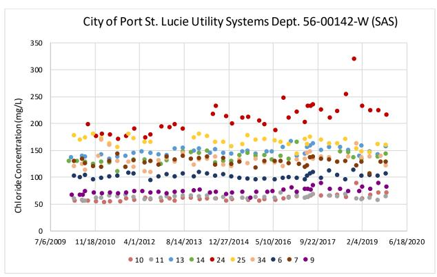
Figure 6-10. Chloride concentration trends at surficial aguifer system wells monitored by the City of Port St. Lucie Utility Systems Department.
