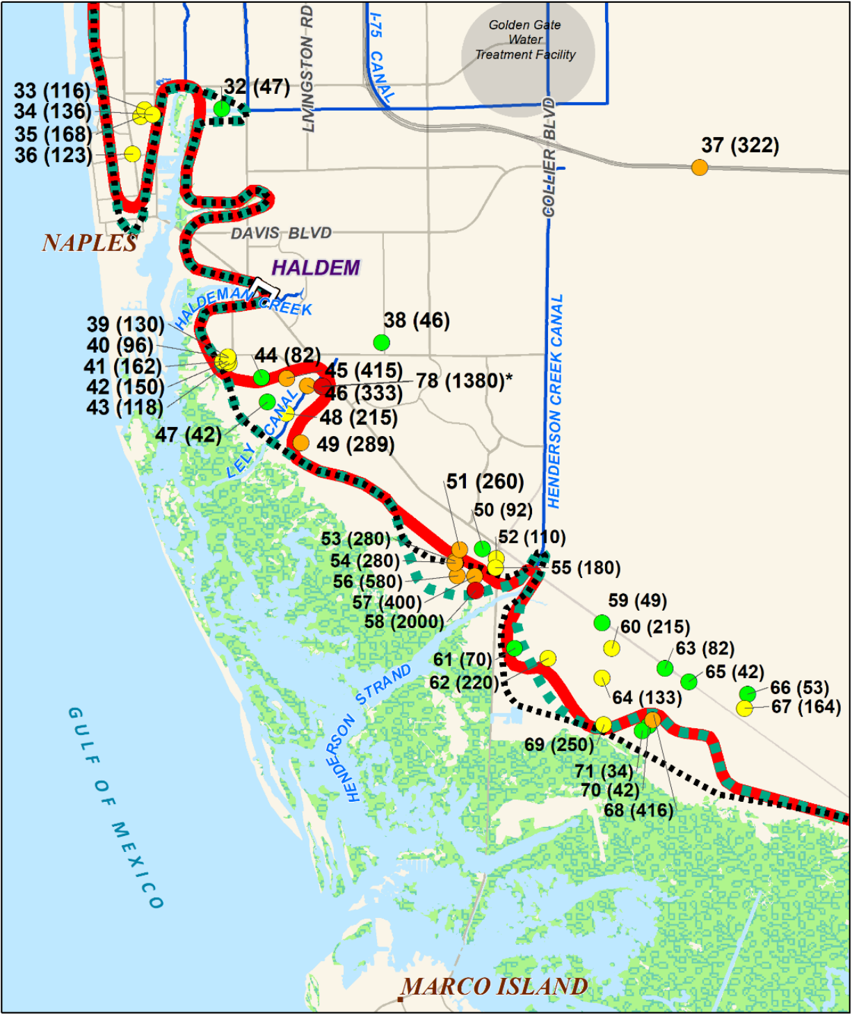
Figure 15. Position of the saltwater interface in the Water Table aquifer in Collier County.
