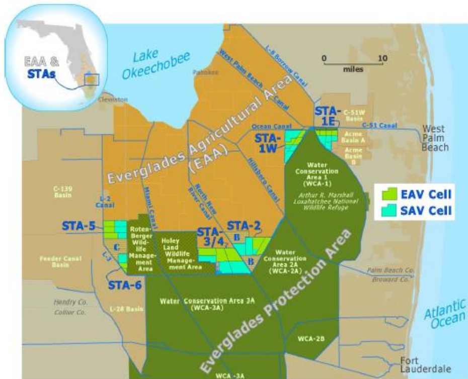
Figure 3-1. Location of the Everglades Stormwater Treatment Areas (STAs) 1 East (1E), 1 West (1W), 2, 3/4, and 5/6 in relation to the Everglades Protection Area, the dominant STA vegetation communities [emergent vegetation (EAV) or submerged aquatic vegetation (SAV)].
