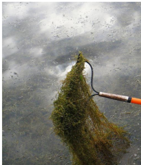
Figure L-2. Rake method of identifying species present at specific sites and their relative density, e.g., 0=absent, 1=sparse, 2=dense, 3=very dense.
