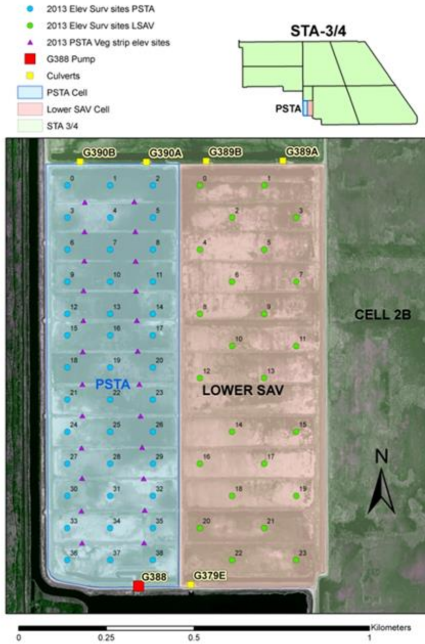
Figure 4-6. PSTA and SAV Cell 2013 elevation survey locations.
