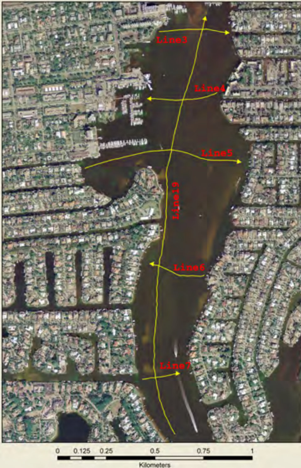
Figure 11. Map showing position of CHIRP seismic tracks within northern Naples Bay. Arrows denote the direction of track portrayed in seismic profiles.
