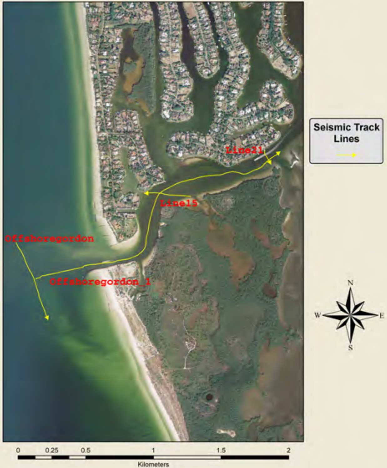
Figure 15. Map showing position of CHIRP seismic tracks within Gordon Pass. Arrows denote the direction of track portrayed in seismic profiles.
