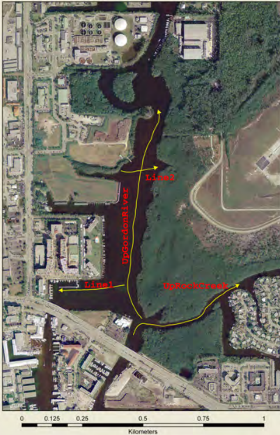
Figure 10. Map showing position of CHIRP seismic tracks within Gordon River and Rock Creek. Arrows denote the direction of track portrayed in seismic profiles.
