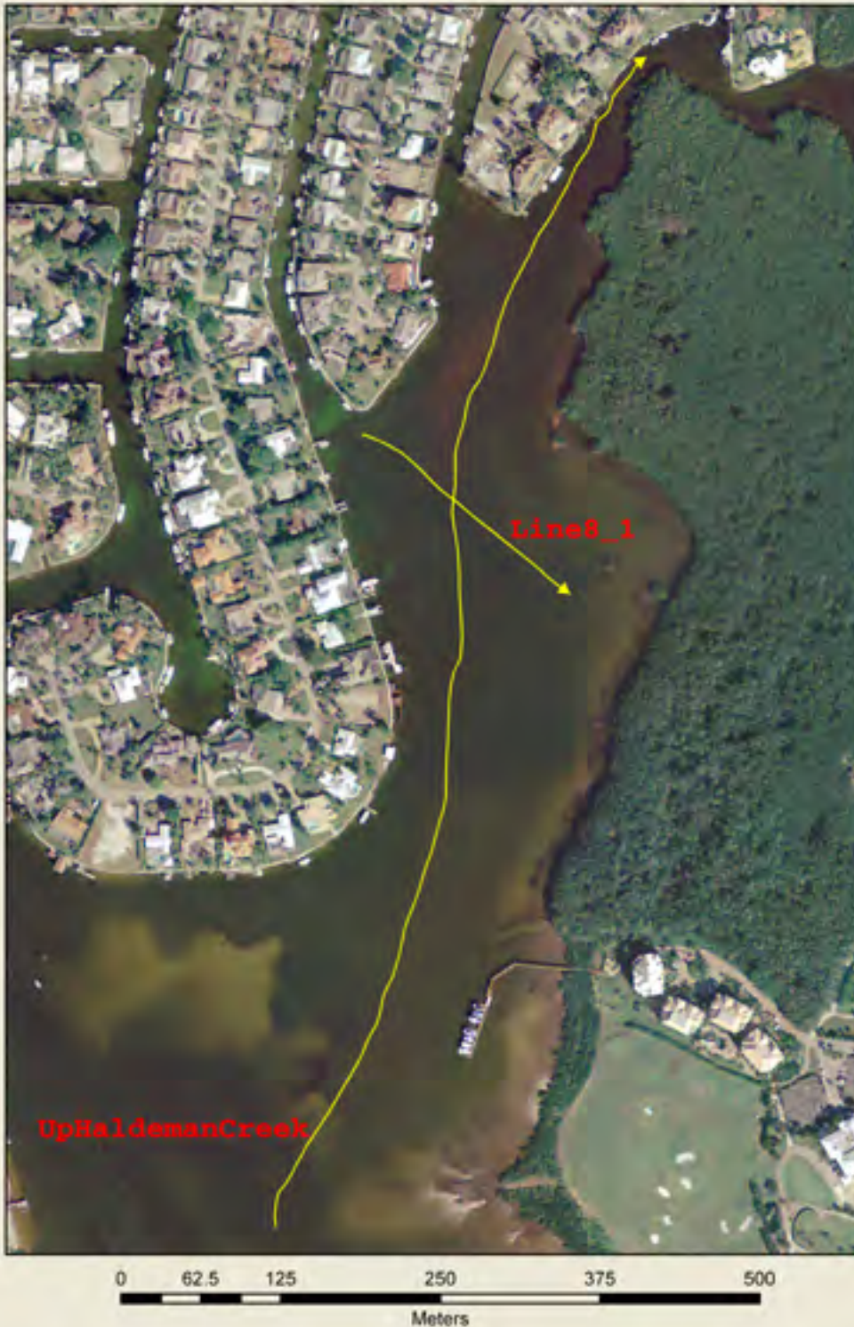
Figure 14. Map showing position of CHIRP seismic tracks within Haldeman Creek. Arrows denote the direction of track portrayed in seismic profiles.
