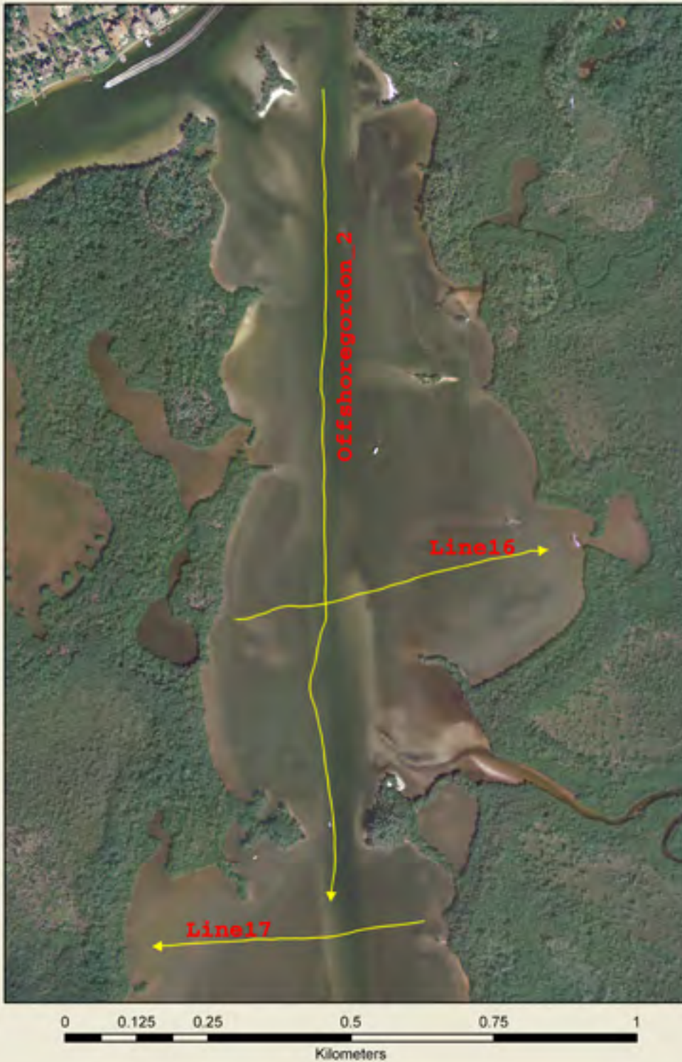
Figure 13. Map showing position of CHIRP seismic tracks within Dollar Bay. Arrows denote the direction of track portrayed in seismic profiles.
