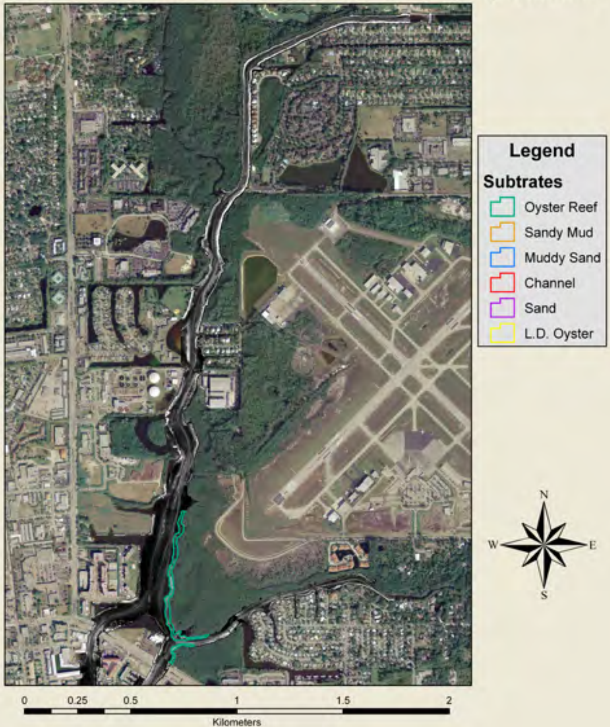
Figure 30. Side-scan sonar mosaic for Gordon River and Rock Creek showing the spatial distribution of the 6 substrate types.
