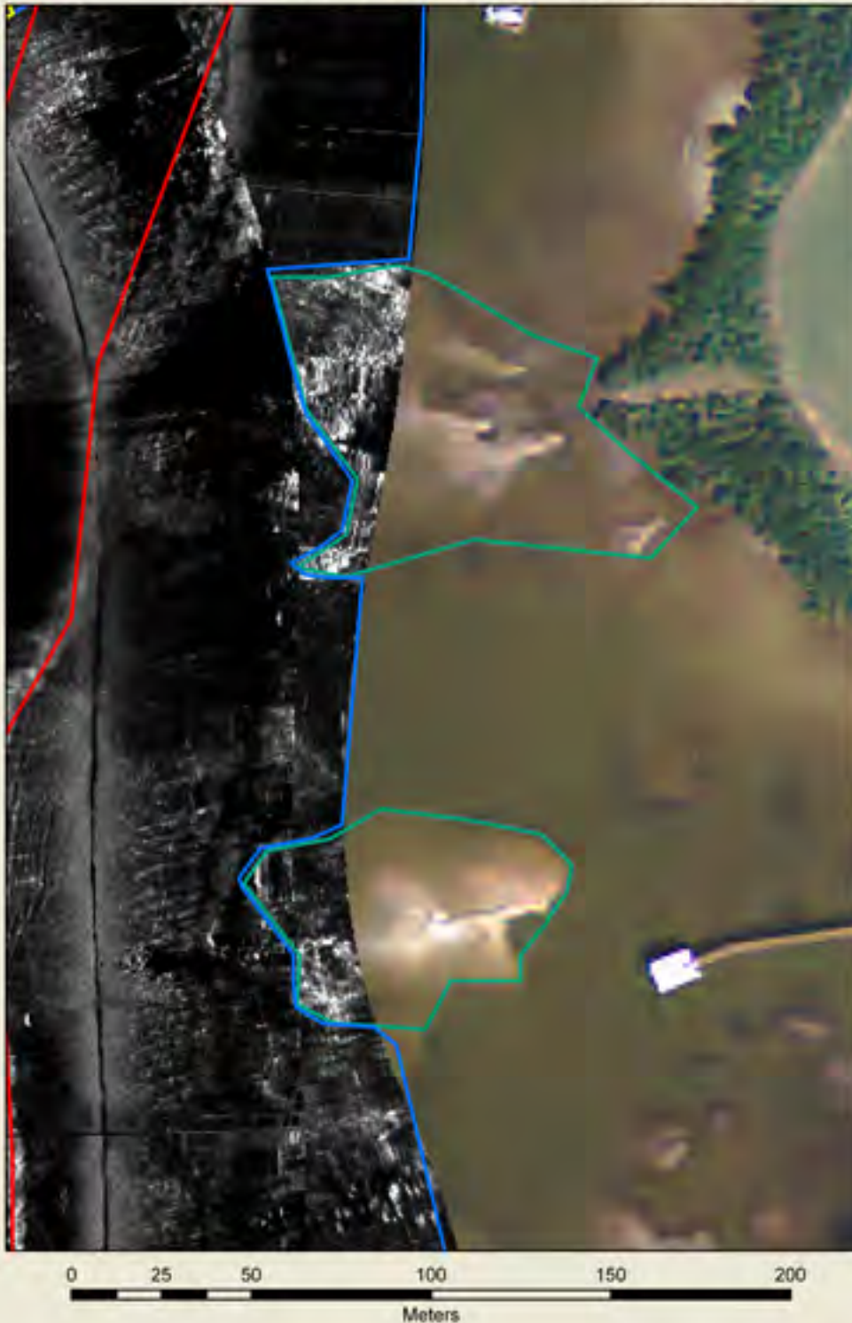
Figure 25. Side-scan sonar mosaic for the region offshore of Winstar, south of Haldeman Creek's mouth, showing the spatial distribution of the 6 substrate types.
