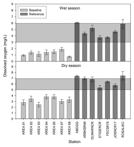
Figure 8-1. Mean ( $\pm$  standard error of the mean) dissolved oxygen (DO) concentrations in free-flowing, blackwater, south Florida streams and remnant runs of the channelized Kissimmee River during the wet (June–November) and dry (December–May) season. Cross-hatched area represents expected range of DO concentrations in the Kissimmee River after restoration.
