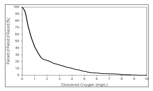
Figure 8-3. Percent of period of record (July 1997–June 1999) that Dissolved oxygen (DO) within remnant river channels exceeded x-axis values. Data are based on mean (average of 96 values per day) daily DO concentrations at two remnant river run stations in Pool C (Oxbow 13 and Montsdeoca Run). Dissolved Oxygen readings were taken at a depth of 1.0 m at each station.
