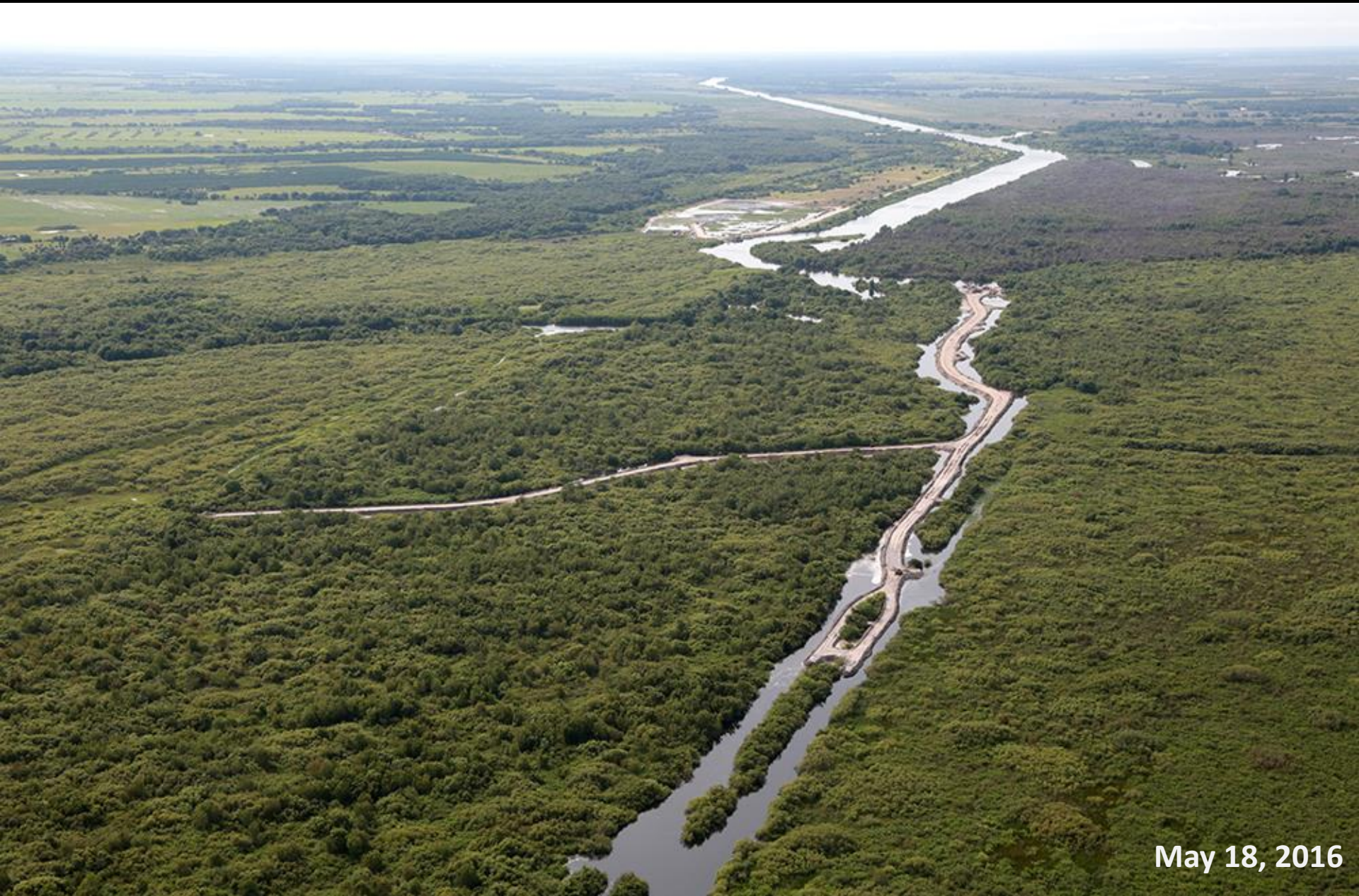
MacArthur Ditch backfill looking south.
