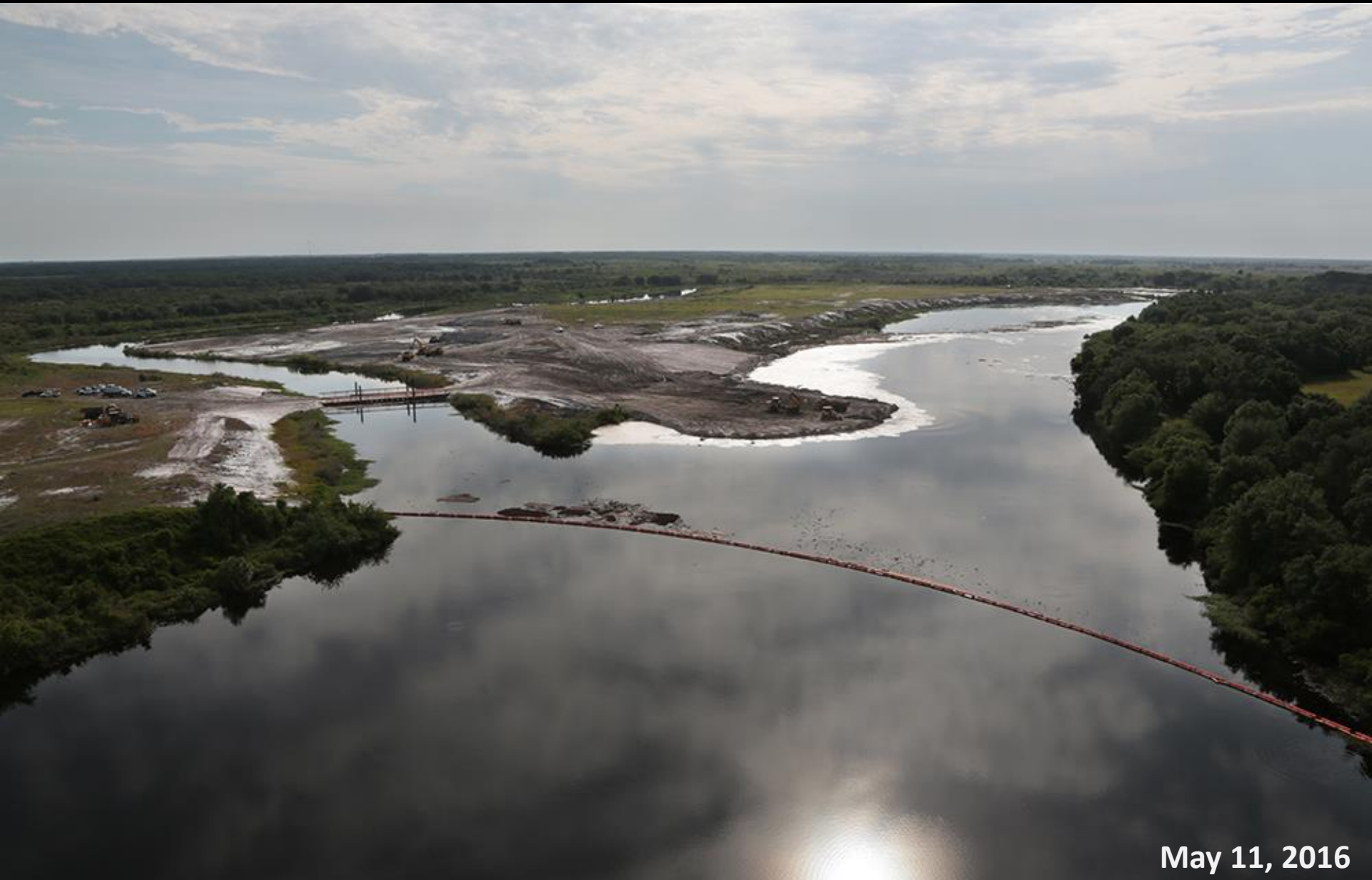
Kissimmee River Reach 3 restoration area looking south down the C-38 where a plug is being placed at the north end of reach 3 just south of the HW98 bridge.
