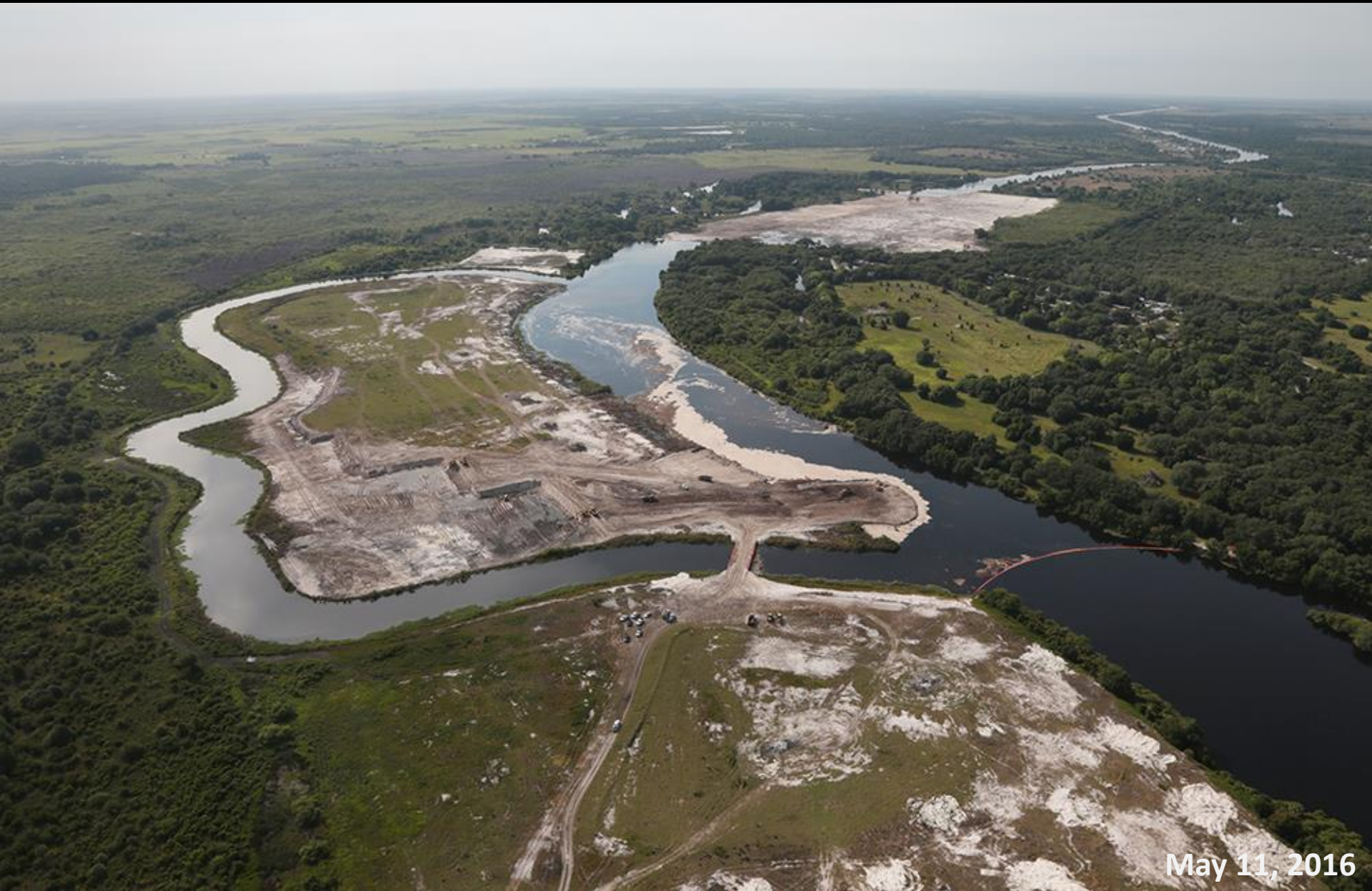
Kissimmee River Reach 3 restoration area looking south up the C-38 canal where a plug is being placed at the north end of reach 3 just south of the HW98 bridge.
