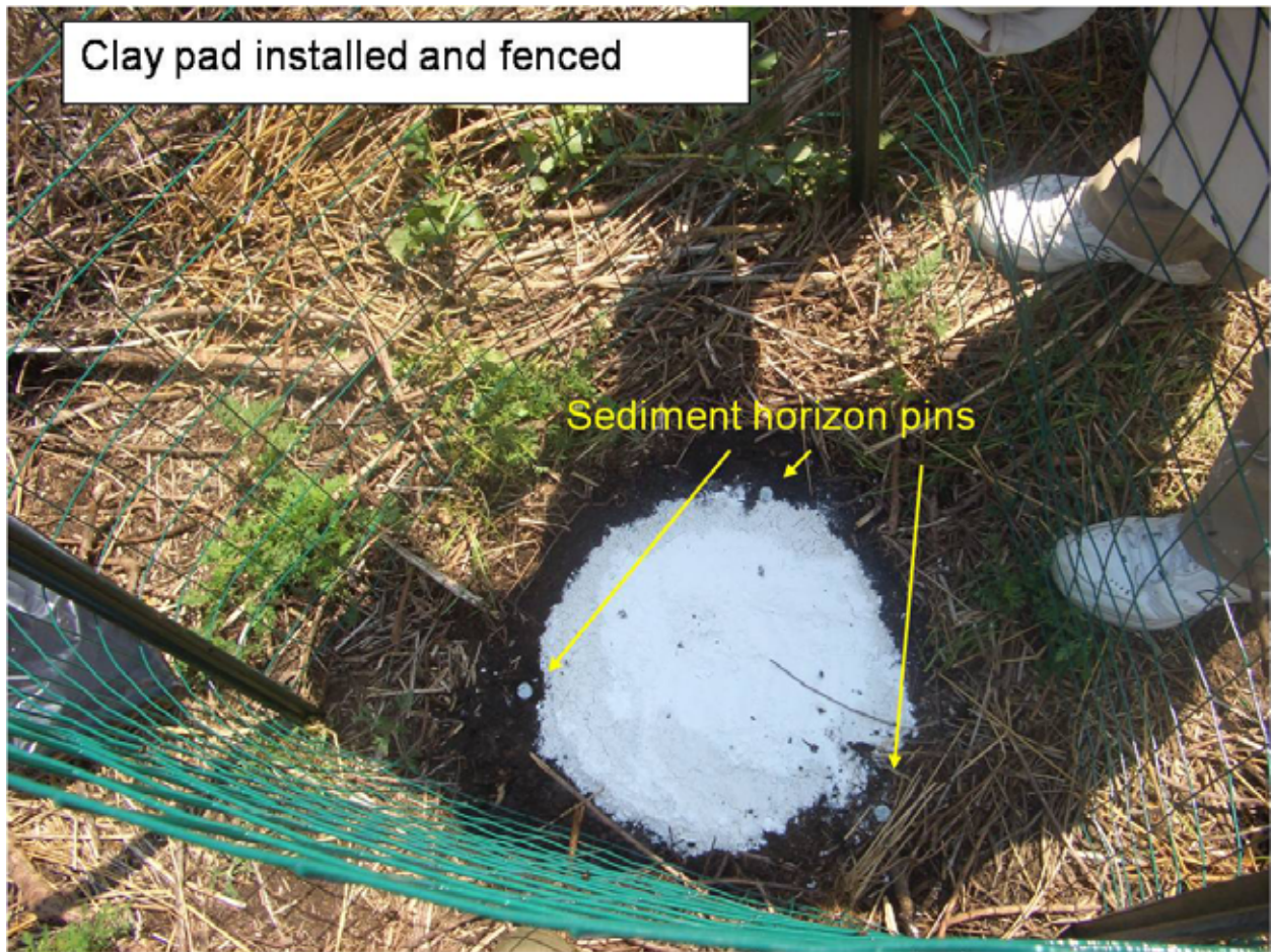
Figure 3-3. Typical feldspar clay pad with associated sediment horizon pins and fenced enclosure. Enclosures were used only in Pool D to prevent disturbance from cows or other grazers. Photo credit: Edward Schenk, USGS.
