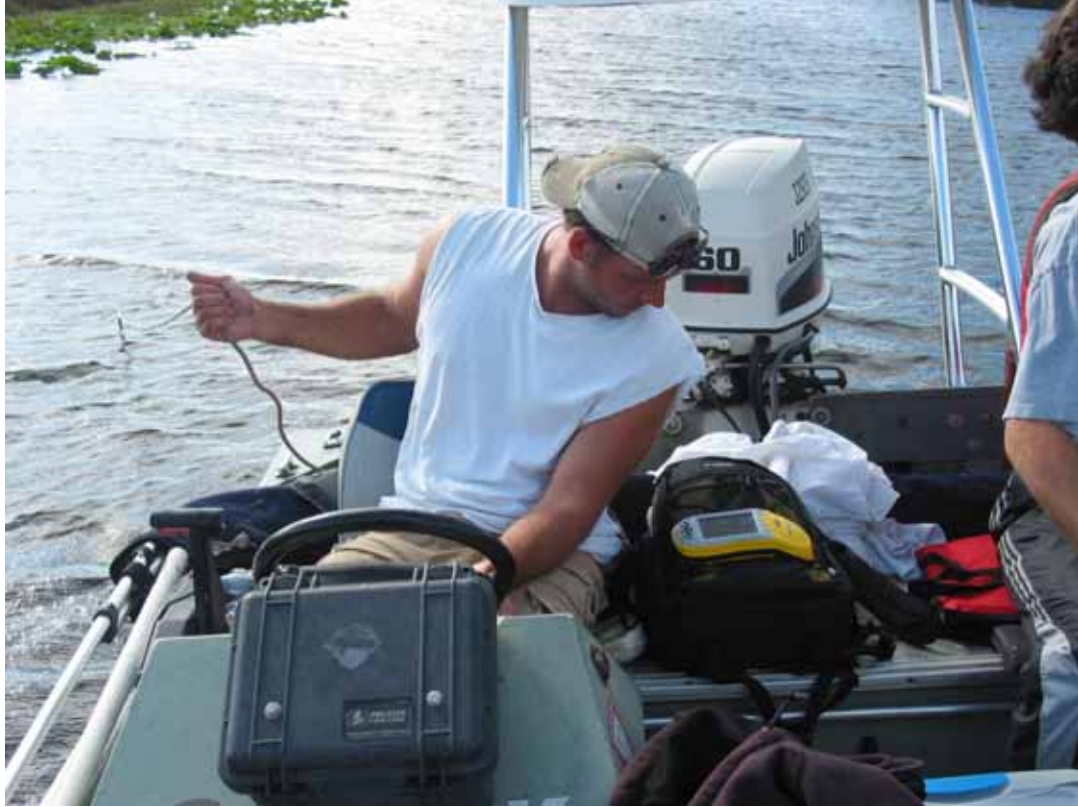
Figure 5-10. Stabilizing the boat with anchor and checking the GPS for randomly selected predetermined coring location.
