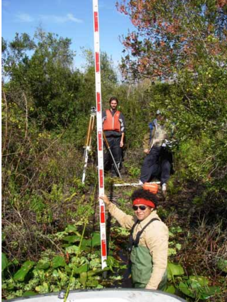
Figure 4-5. Survey methods using survey rod, level and rope along designated river transects. This photograph was taken in January 2009 in Persimmon Mound Run in Pool A.
