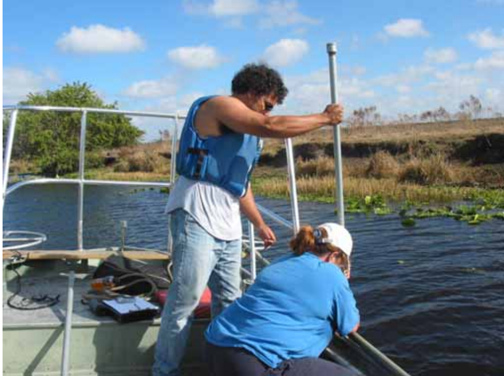
Figure 5-8. Coring the streambed with vacuum piston corer. Photograph shows galvanized pipe extension.
