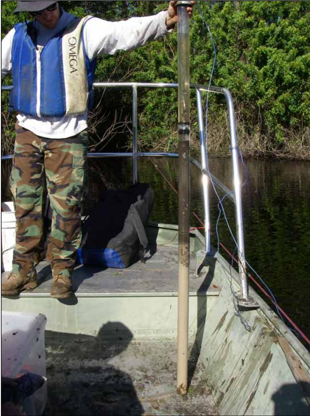
Figure 5-6. This photograph shows the length of polycarbonate tubing and how the bottom sediments of the Kissimmee River can be described. In this core, organic and fine sediments overlie a sand bottom, presumably the bed of the channel prior to channelization.
