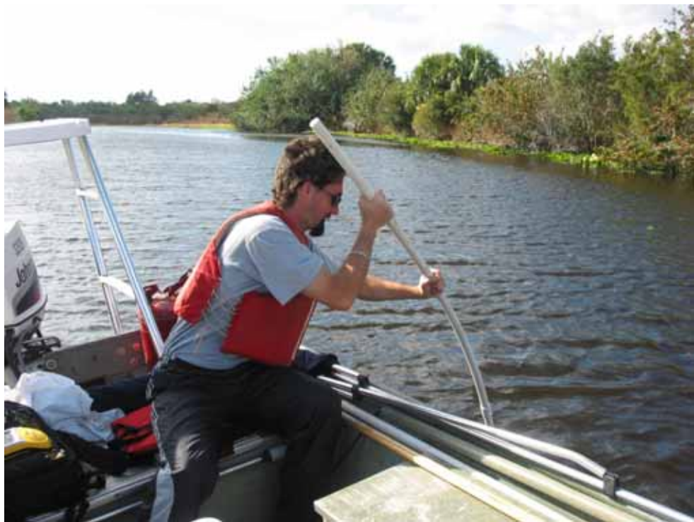
Figure 5-8. Coring the streambed with vacuum piston corer. Photograph shows galvanized pipe extension.
