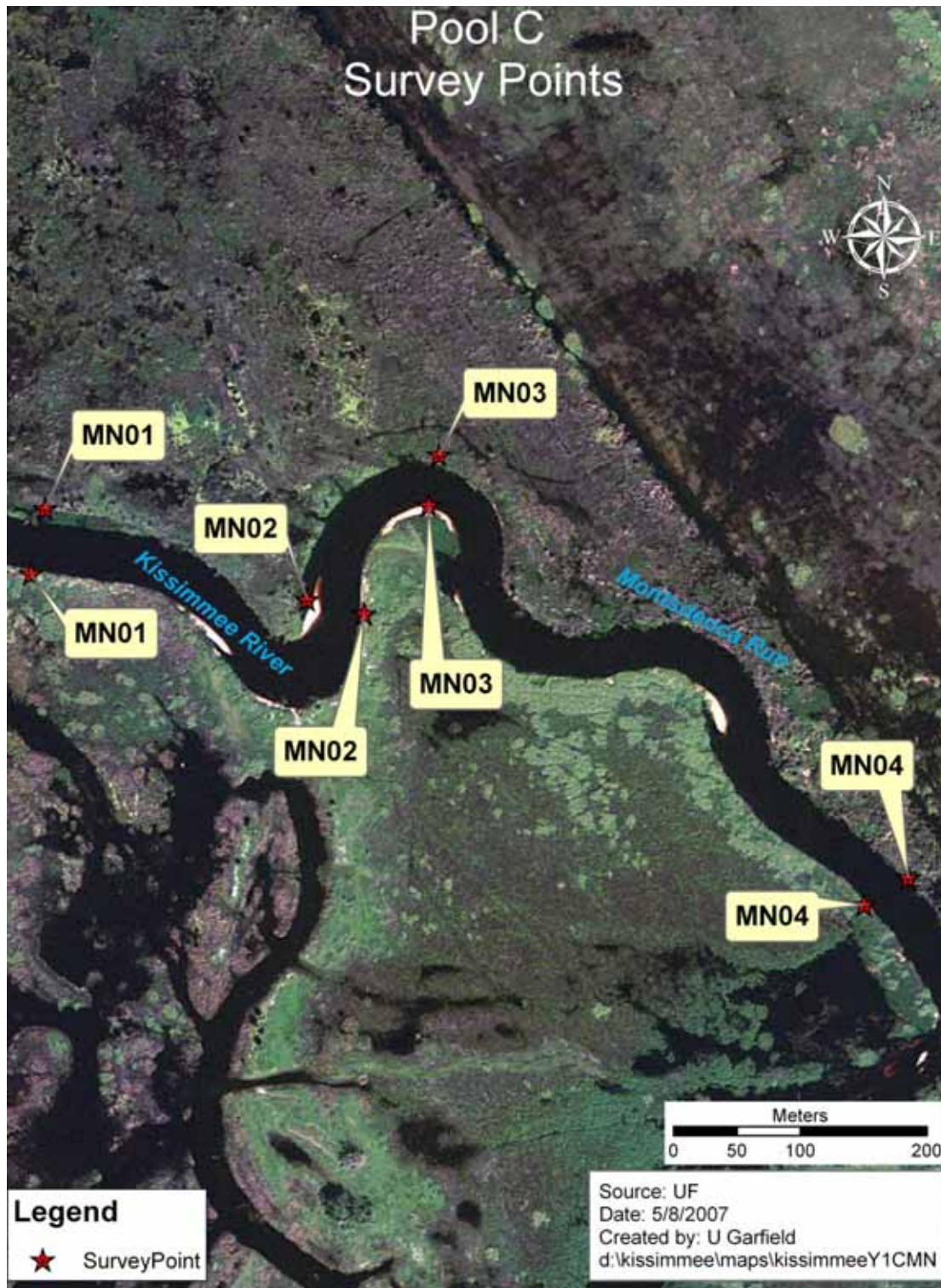
Figure 4-9. Transect locations in Montsdeoca Run, Pool C. Transects 1 and 4 are considered straight reaches and Transects 2 and 3 are bendways located across the bar apex.
