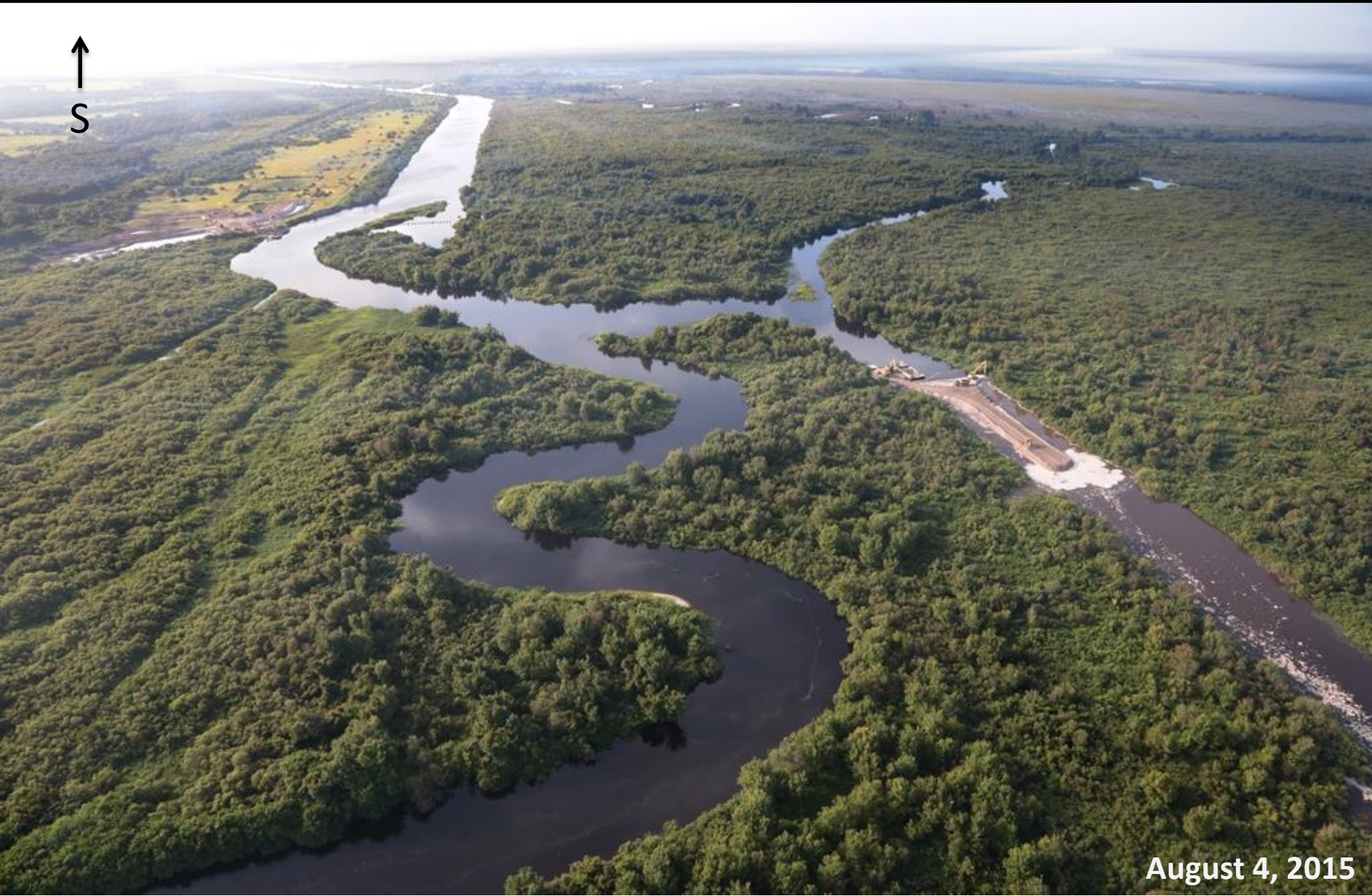
Looking south at construction of the MacArthur Ditch contract. A spoil plug has been placed on the south end of the ditch and the backfill continues northward into the Kissimmee River Restoration Phase I restoration area floodplain.
