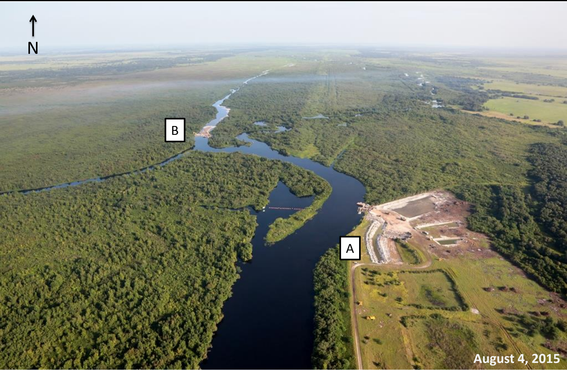
Looking north at construction of the MacArthur Ditch contract (B) and borrow site (A): The backfill continues northward into the Kissimmee River Restoration Project Phase I restoration area floodplain.
