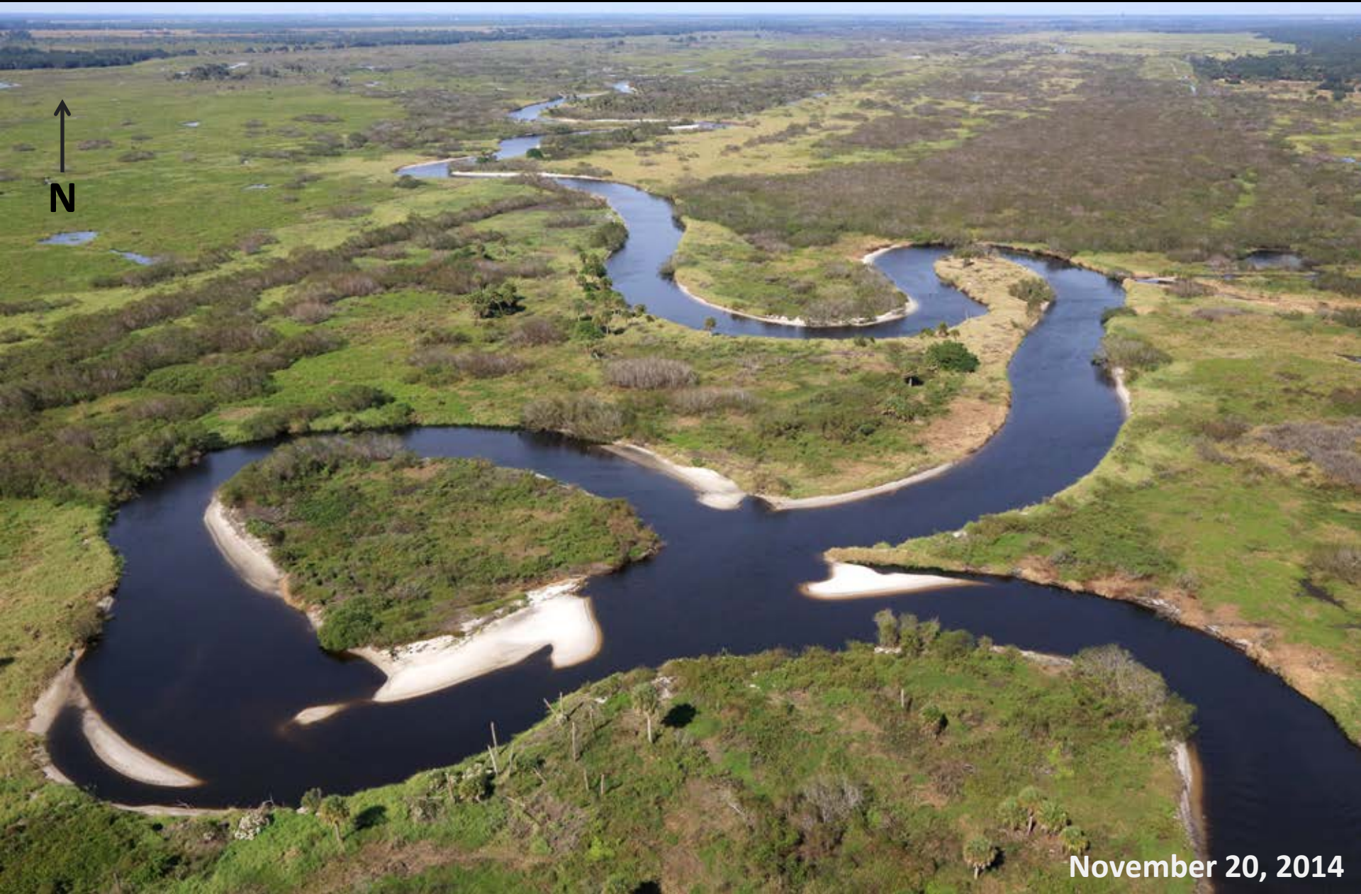
Micco breakthrough under lower discharge exposes sand deposits resulting from both the former and new routes that flow has taken. (Discharge was ~300 cfs for about 6 weeks prior to this photo.)
