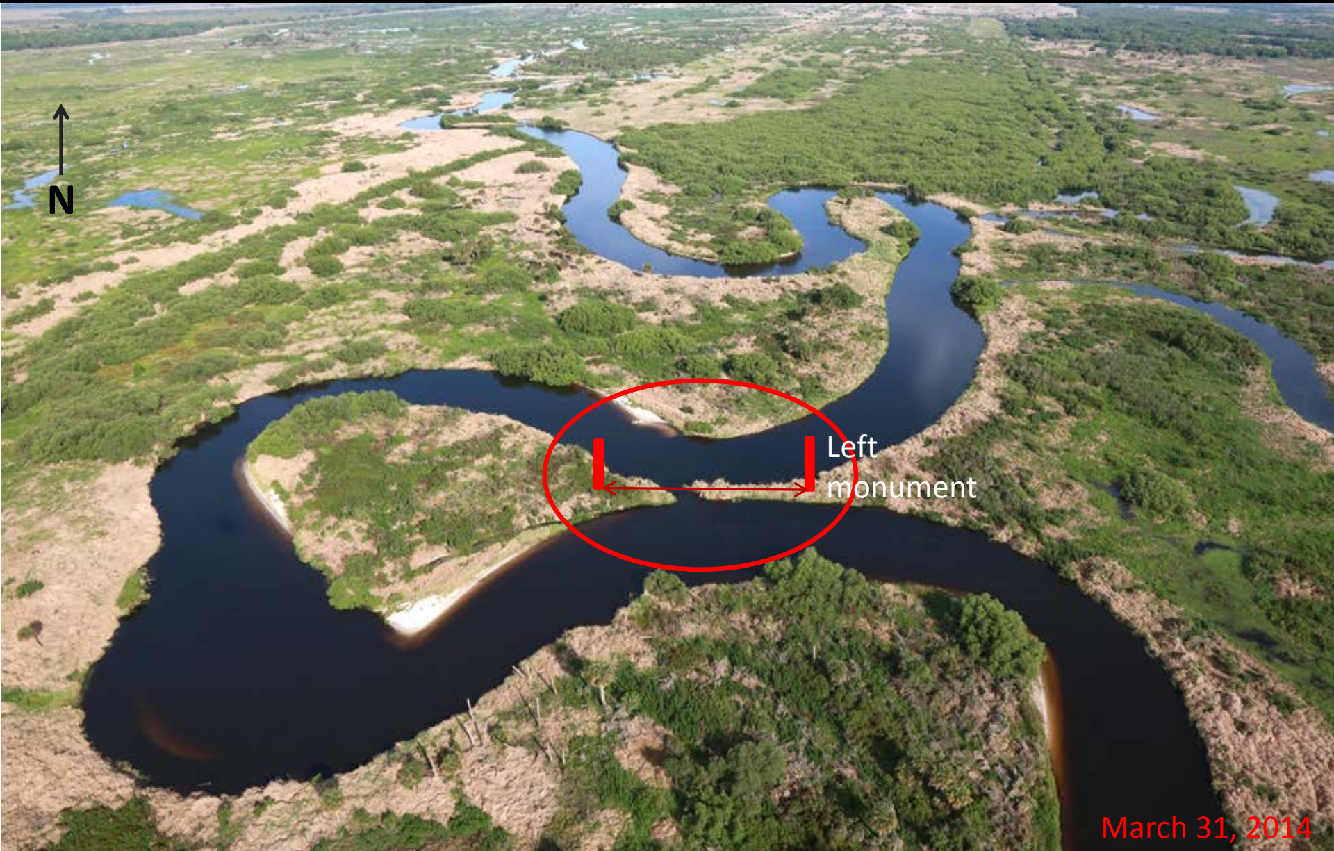
The beginning formation of a meander cutoff in Micco Run in the Kissimmee River. The cutoff formed sometime in the two weeks prior to the photo date and may ultimately form an oxbow lake. A cross-section survey transect was set up to capture monthly changes in the cutoff channel.
